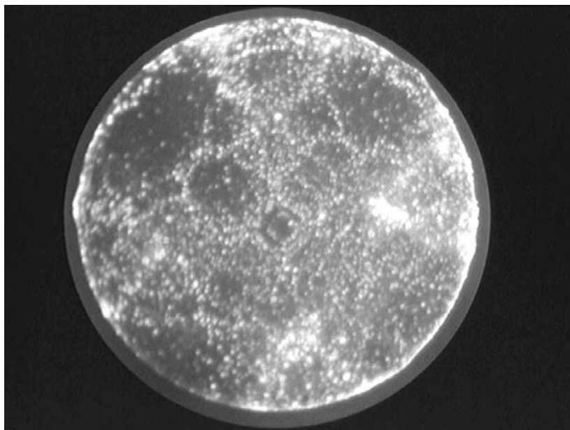
Fig. 2. FIM pattern of the clean palladium surface
