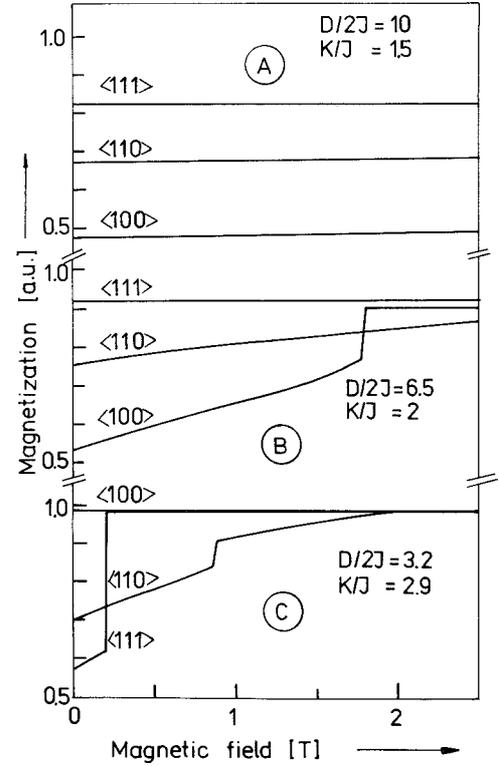
Fig. 4. Magnetisation along the principal axes predicted by spin model for three selected values of the crystal field and the exchange anisotropy (ref. [25]).
