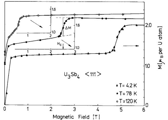
Fig. 5. Magnetisation curves for  $\text{U}_3\text{Sb}_4$  along the  $\langle 111 \rangle$  axis at three different temperatures (ref. [26]).
